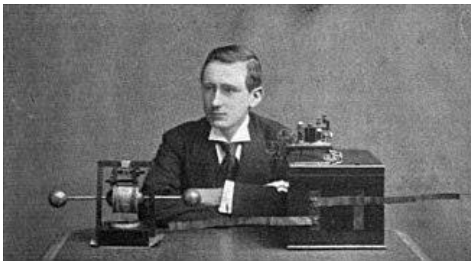
Publicity photo of Marconi and his spark-gap transmitter and receiver, 1897
